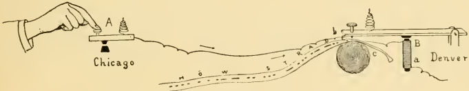
HOW A MESSAGE BY TELEGRAPH IS SENT. 2
